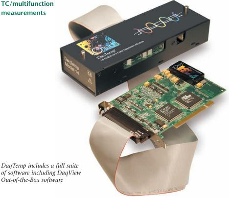
DaqTemp is derived from the PC; therefore no external power supplies or transformers are needed.
