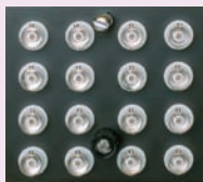
BNC termination panel (DBK602) features 16 BNC connectors
