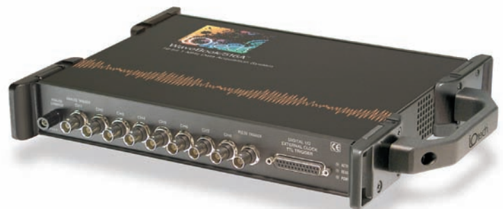
WaveBook/516A includes a parallel port for connecting to the WaveBook/516E
