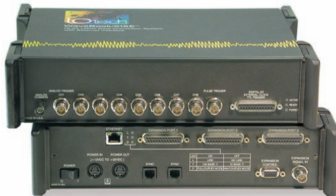
The WaveBook/516E includes a 10/100BaseT Ethernet interface
